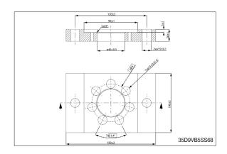
(2) Assembly tool for dust seal Material: Free cutting steel
