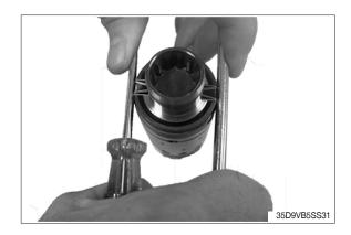
(6) Mount ring (10) on sleeve. Ring should move freely independent from spring.
