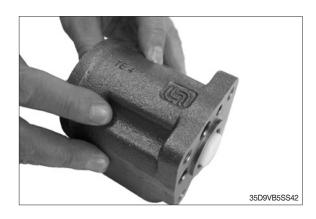
(18) Put steering unit housing on assembly fastening device toward the tip of steering column. Insert ball (3) into indicated hole.
