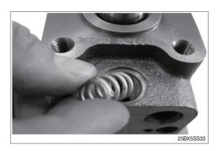
(33) Mount O-ring on adjusting screw (30), and fasten the screw with 6-mm Allen key. Set pressure on test panel in accordance with valve setup specifications.
