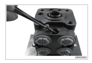
(5) Make use of 5-mm Allen key to remove adjusting screw (25) mounted with O-ring (40).
