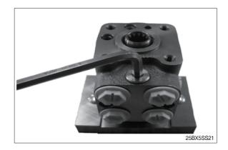
(2) Make use of 6-mm Allen key to remove adjusting screw (30).
