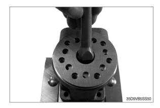
(26) Mount 2 O-rings (18) on gear wheel set (17), and put the set on cardan shaft (13). Align holes of gear wheel set with those of housing thread.
