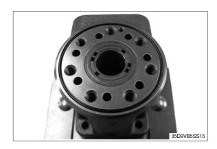
(16) Make use of Torx bit of size T50 to remove check valve (37).
