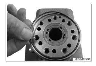
(24) Put distributor plate (16) on housing while aligning with thread holes.
