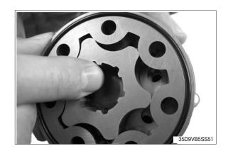
(27) Put end cover (19) on port while ensuring that product code is positioned parallel with port.
