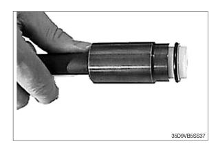
(13) Insert assembling tool into the bottom of steering unit.
