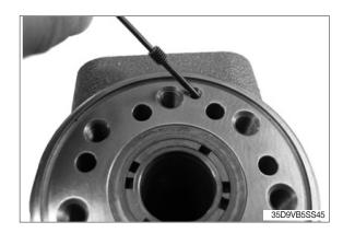
(21) Insert ball (33) into two indicated holes respectively.
