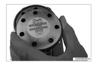
(11) Lift gear wheel set (17) up, and remove 2 O-rings (18).
