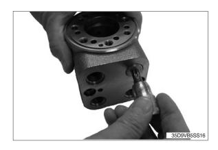
(17) Shake housing to take check valve ball (3) and ball (36) out of housing.
