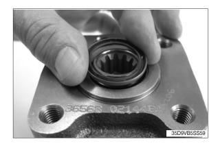
(40) Make use of tools and mallet for assembling dust seal to mount dust seal ring (1).
