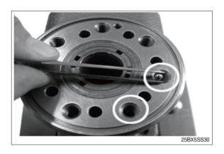
(22)Insert pin (34) into 2 identical holes respectively.
