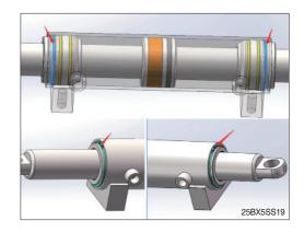
(5) Move piston rod several times for ensuring max. stroke. Mount O-rings and seals correctly before hydraulic oil plays on cylinder.
