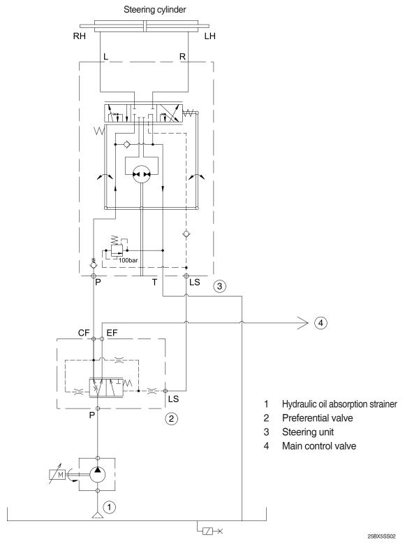
Hydraulic oil is supplied from hydraulic pump to preferential valve. When driver turns steering wheel, hydraulic oil is supplied first to steering unit by working circuit inside preferential valve. Hydraulic oil inside steering unit is expanded or shrunk, and then supplied to steering cylinder of forklift truck. hydraulic oil excessively discharged from hydraulic pump flows to hydraulic oil tank along main control valve and preferential valve EF port.
