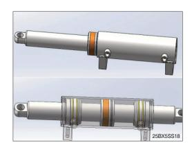
(4) Mount snap ring (13) on tube assembly (12) groove. Move piton rod (16) to the limited position. Mount circlip.
