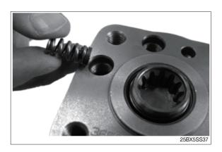
(37) Mount O-ring (40) on adjusting screw (25). Make use of 5-mm Allen key to fasten adjusting screw. Set pressure on test panel in accordance with valve setup specifications.
