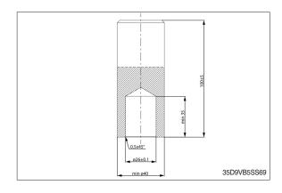
(3) Tool for shaft seal, O-ring, rotor glide Code: 11092408.
