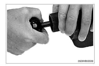
(15) Withdraw assembling tool from steering unit.
