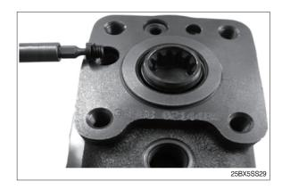
(9) As shown on the figure, turn steering unit up side down, and put in on fastening tool. Make use of 13-mm ring or wrenches, remove screws (22, 23) and washer (20).
