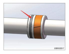
(3) Make use of tool to fasten piston rod (16), and insert piston rod into tube assembly (12). Mount rod covers (15) on the both sides of tube assembly.
