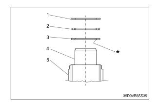
(11) Put steering unit housing on worktable. Prepare assembling tools for mounting shaft seal (5) on spool and sleeve set (2).
