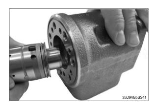
(17) Assembling tool is pulled out of spool assembly, and shaft seal (5) is mounted.
