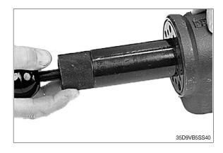
(16) Assemble spool and sleeve assembly on cross pin (11) in parallel direction while rotating the assembly a little.
