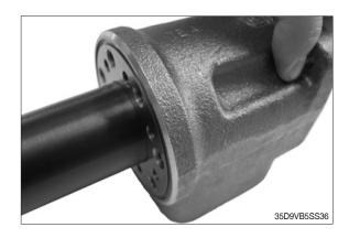
(10) Lubricate shaft seal (5) with hydraulic oil, and put it on tool. Make sure that shaft seal (5) is correctly positioned on insertion tool.
