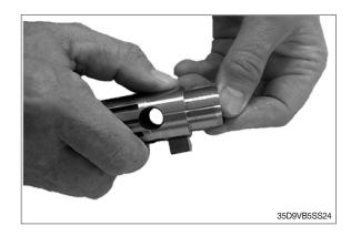
(24) Make use of screw driver to carefully remove dust seal ring (1) and shaft seal (5).
