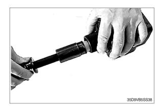
(14) Press the tool into housing, and rotate shaft seal (5).
