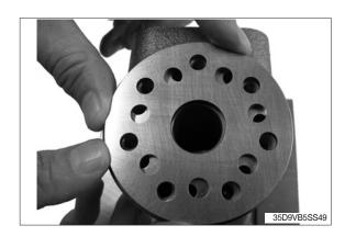
(25) Put cardan shaft (13) inside slot for connecting circumference port, and aligning cross pin (11).
