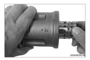
(19) Remove bearing assembly (7) from spool and sleeve (2). Outer bearing may be caught inside housing. Make sure that bearing is normally pulled out.
