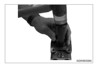
(41) Once assembling is complete, install plastic plugs for keeping inside of port clean.
