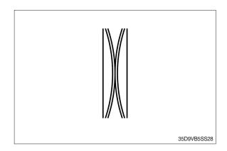
(3) Spool and sleeve set for steering unit should precisely be aligned to each other for mounting., Small marks are on the nearest slot of spring set, and all of sleeves. There are no marks on most of spools and sleeve sets. They are arranged facing each other on 1 of 2 available locations.
