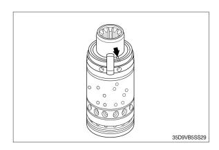
(4) Mount spool on sleeve, and make sure that leaf spring (12) is mounted on slot.
